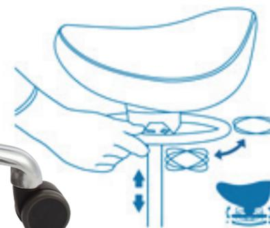
*The ring easily turns clockwise & counter-clockwise to increase or decrease the amount of dynamic motion of the seat. I found adjusting the seat to be very simple.*
