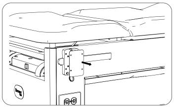
3. Attach new mounting plate cover to mounting plate using four new push rivets.
