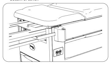
15. Attach lock socket to beam.
