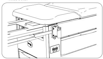
14. Attach handle support cover to handle support using three new large push rivets, one on top and two on bottom of cover.
