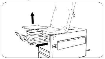
5. From inside of cabinet loosen three hex head bolts attaching mounting plate. Pull plunger downward and remove mounting plate.
