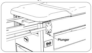
11. Attach mounting plate cover to mounting plate using four new small push rivets.
