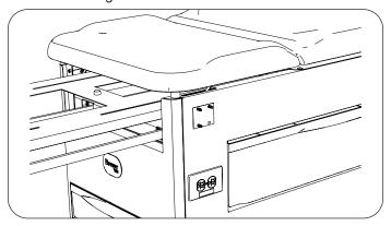
9. Position beam against glide. Round end of beam faces forward, and set screws face downward.
