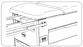
10. Pull plunger downward. Position groove in mounting plate over beam and thread/tighten three hex head screws into mounting plate.
