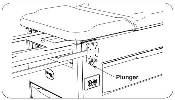
13. Attach handle support to mounting plate using four hex head bolts.
