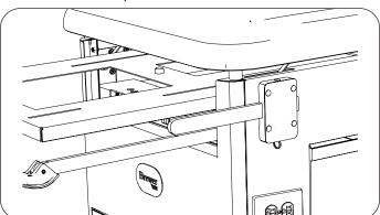
12. Attach lock socket to beam.
