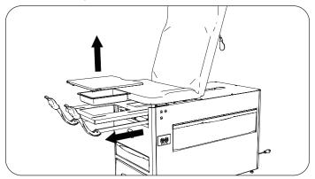
7. From inside of cabinet loosen three hex head bolts attaching mounting plate. Pull plunger downward and remove mounting plate.
