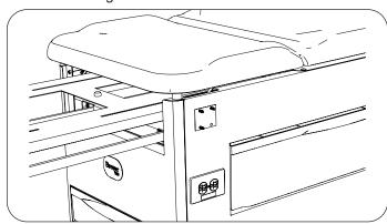
11. Position beam against glide. Round end of beam faces forward, and set screws face downward.
