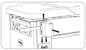
5. Remove four hex head bolts attaching handle support to mounting plate. Remove handle support.
