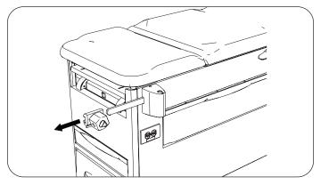
Using supplied pry bar, remove three push rivets attaching handle support cover to handle support, one on top and two on bottom of cover. Remove cover.
