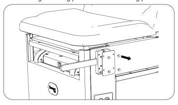
4. To gain access to inside of cabinet, pull out stirrups (if equipped) and leg extension. Remove upholstered pad and debris pan.
