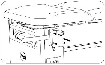
4. Remove plunger from mounting plate using 1/4" open end hex wrench. Discard plunger.
