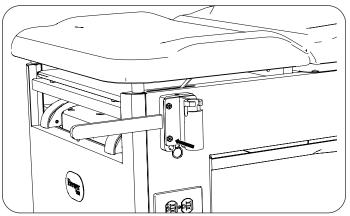
7. Attach handle support cover to handle support using three large push rivets, one on top and two on bottom of cover.
