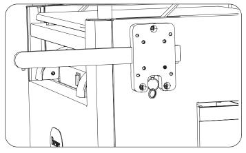
4. Attach mounting plate cover to mounting plate using four small push rivets.
