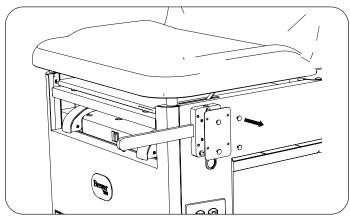
2. Remove plunger from mounting plate using 1/4" open end hex wrench. Discard plunger.
