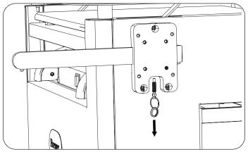
3. Install new plunger using 1/4" open end wrench.
