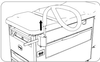
2. Using supplied pry bar, remove three push rivets attaching handle support cover to handle support, one on top and two on bottom of cover. Remove cover.
