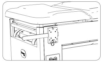
6. Attach handle support to mounting plate using four hex head bolts.
