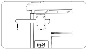
9. Attach lock socket to beam.
