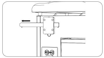
4. Remove stop screw from front of beam using provided 7/64" Allen wrench.
