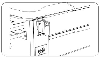
8. Attach handle support cover to handle support using three large push rivets, one on top and two on bottom of cover.
