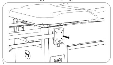
Pull plunger downward and install beam in new mounting plate. Round end of beam faces forward and set screws face downward. Position new mounting plate and thread/tighten three hex head screws into mounting plate.
