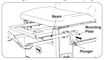
Pull plunger downward and install beam in new mounting plate. Round end of beam faces forward and set screws face downward. Position mounting plate and thread/tighten three hex head screws into mounting plate.
