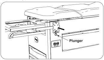
9. Attach handle support to mounting plate using four hex head bolts.
