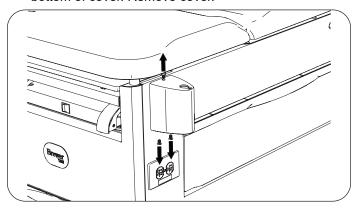
3. Remove four hex head bolts attaching handle support to mounting plate. Remove handle support.
