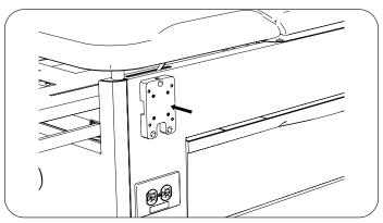
7. Attach handle support to mounting plate using four hex head bolts.
