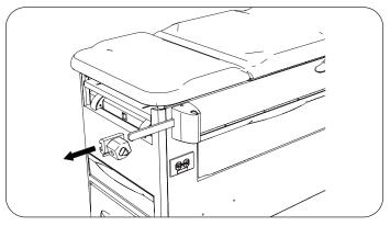
4. Using supplied pry bar, remove three push rivets attaching handle support cover, one on top and two on bottom of cover. Remove cover.
