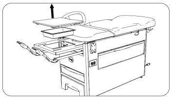
5. Remove mounting plate by loosening three hex head bolts from inside of cabinet. Discard mounting plate.
