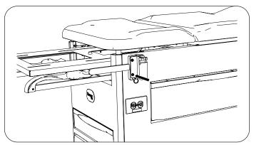
10. Attach handle support cover to handle support using three large push rivets, one on top and two on bottom of cover.
