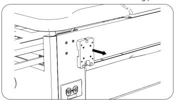
6. Position new mounting plate and thread/tighten three hex head screws into new mounting plate.
