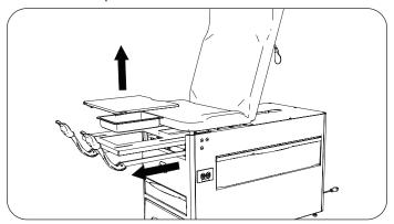
From inside of cabinet loosen three hex head bolts attaching mounting plate. Remove mounting plate and beam. Pull plunger downward and remove beam from mounting plate. Discard mounting plate with plunger.
