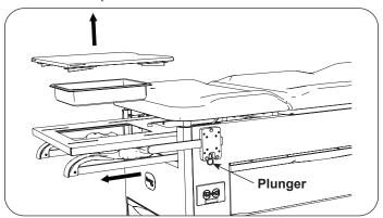
Remove mounting plate and beam by loosening three hex head bolts from inside of cabinet. Pull plunger downward and remove beam from mounting plate. Discard mounting plate with plunger.
