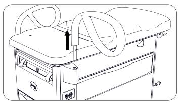
Using supplied pry bar, remove three push rivets attaching handle support cover, one on top and two on bottom of cover. Remove cover.
