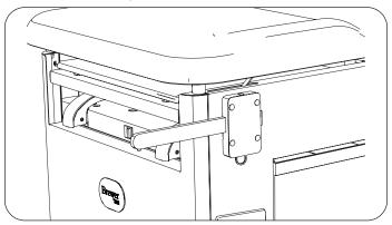
8. Attach lock socket to beam.
