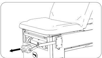
3. Using supplied pry bar, remove four small push rivets attaching mounting plate cover to mounting plate.
