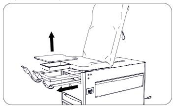
2. Remove three push rivets from cabinet by using provided pry bar, or punching rivets out from the inside of the cabinet.
