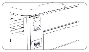
5. Install assist handle support to mounting plate using four hex head screws. Orient support as shown.
