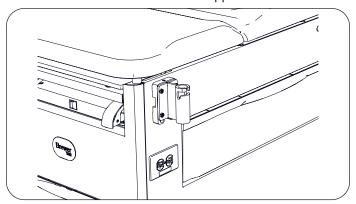
6. Attach assist handle support cover to assist handle support using three push rivets, one on top and two on bottom of cover.
