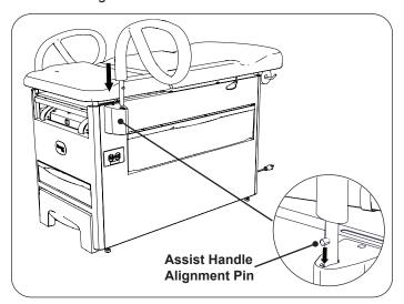
10. The patient assist handles have two locating positions: one rearward and one forward. Position the handle at the desired location and the bar will fall into a detent.
