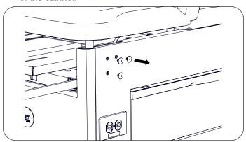
3. From the inside of table, place three hex head screws through holes in cabinet.
