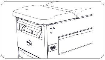
4. Position mounting plate over screws and tighten screws from the inside. Orient mounting plate as shown.
