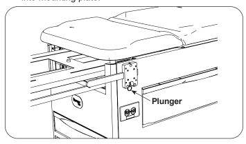
7. Attach assist handle support (provided with assist handle kit) to mounting plate using four hex head screws (provided with assist handle kit).
