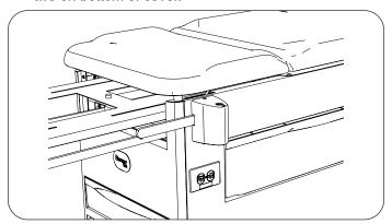
9. Attach lock socket to beam.
