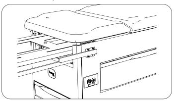
6. Pull plunger downward. Position groove in mounting plate over beam. Thread/tighten three hex head screws into mounting plate.
