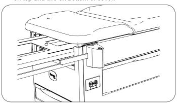
13. Attach lock socket to beam.
