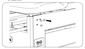
3. Place three hex head screws through holes from inside of cabinet.
