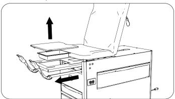
Remove three push rivets from cabinet by using provided pry bar, or punching rivets out from the inside of cabinet.
