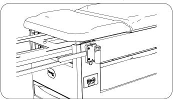
12. Attach new assist handle support cover to assist handle support using three new large push rivets, one on top and two on bottom of cover.
