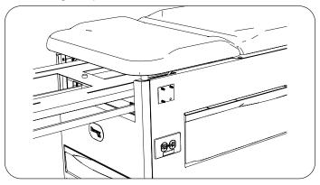
9. Position beam against guide pad. Round end of beam faces forward, and set screws face downward.
