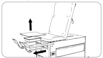
2. Remove three push rivets from cabinet by using provided pry bar, or punching rivets out from the inside of cabinet.
