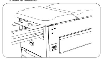
8. Install guide pad over screws.
