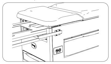
10. Pull plunger downward. Position groove in mounting plate over beam. Thread/tighten three hex head screws into mounting plate.
