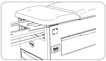
5. Position beam against guide pad. Round end of beam faces forward, and set screws face downward.
