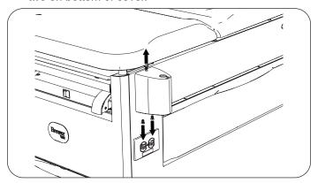
3. Remove assist handle support by removing four hex bolts. Keep support and bolts for reinstallation.
