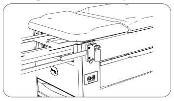
8. Attach assist handle support cover to assist handle support using three large push rivets, one on top and two on bottom of cover.
