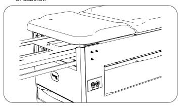
4. Install guide pad over screws.
