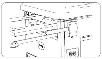
8. Attach lock socket to beam.
