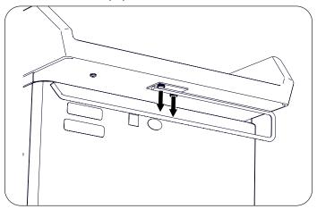
2. Attach new paper roll holder in desired orientation with two new thumb screws.
