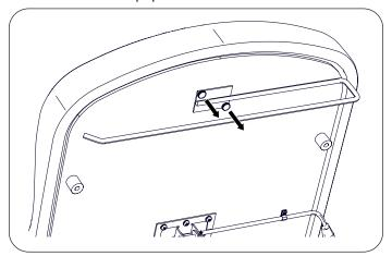
2. Attach new paper roll holder in desired orientation with two new thumb screws.
