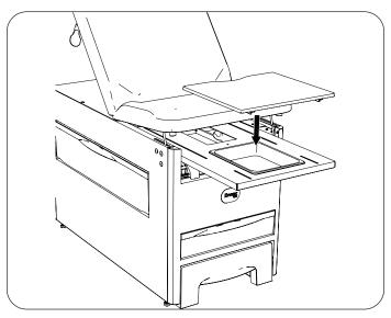
2. Move the toe board back and forth to ensure the board is fully seated.
