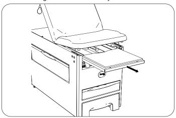
Remove the toe board from the leg extension and discard
