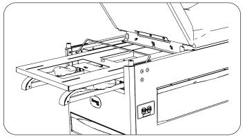
3. With a Phillips screwdriver, reach through the debris pan opening and remove the two pelvic tilt screws.
