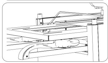
3. Reinstall debris pan and upholstered pad.
