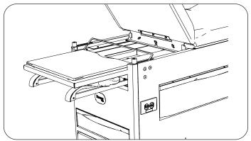
4. Return leg extension and stirrups (if equipped) to stowed position.
