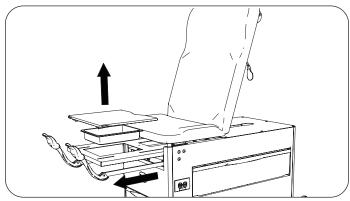
2. Lower back upholstery and raise seat. Do not allow seat to lay rearward onto backrest or the upholstery may tear. Prop seat in raised position (prop not shown).
