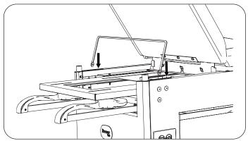
2. Fasten and tighten new pelvic tilt bar using two new screws provided.
