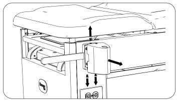
3. Remove four hex head bolts attaching handle support to mounting plate. Remove handle support and discard.
