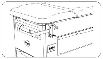
5. Attach handle support cover to handle support using three new push rivets, one on top and two on bottom of cover.
