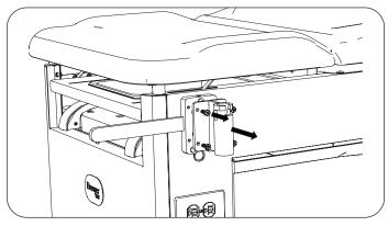
4. Attach new handle support to mounting plate using four hex head bolts.
