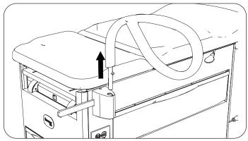
2. Using supplied pry bar, remove three push rivets attaching handle support cover to handle support, one on top and two on bottom of cover. Remove cover.
