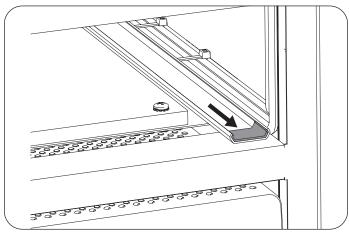
2. Place the drawer into the drawer opening. Align the drawer slides with the glide tracks.
