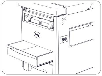
2. While facing the table reach below the drawer to locate the locking tabs. Push both tabs to the left and pull on drawer to remove it. Discard drawer. The illustration below shows a close-up of the locking tab.
