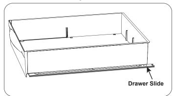
3. With the drawer angled slightly upward, push the drawer into the table.
