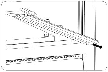
3. Locate the tab on the bottom side of the new drawer slide and the cut-out at the rear of the drawer opening. Insert the tab on the new drawer slide into the cut-out in the cabinet.
