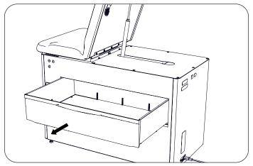
2. Insert drawer dividers into coordinating divider ribs, making sure small hole in the divider is on the bottom.
