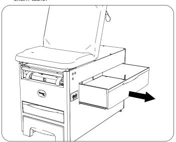
6. Drill out the rivets on both drawer slides.
