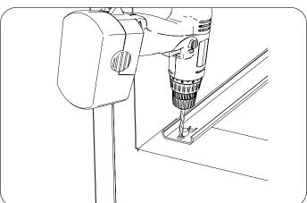
7. The right side ends of the drawer slides have a tab that seat into a slot in the cabinet. Pull the entire rear drawer assembly out of the exam table and discard.
