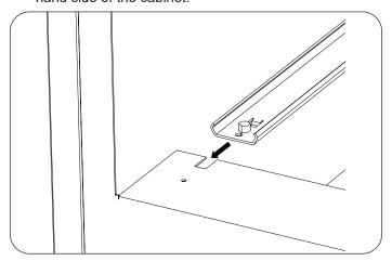
Carefully push the drawer further into the cabinet and align the mounting holes in the drawer slides with the holes in the cabinet. You may need to adjust the drawer slides slightly for proper alignment. 4. Secure each end of the drawer slides with the four screws and hex nuts provided.
