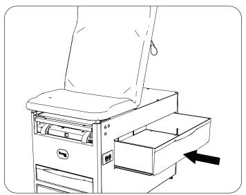
2. Guide the drawer slide tabs into the slots on the right hand side of the cabinet.
