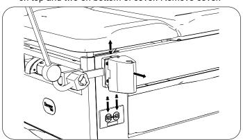
3. Install new handle support cover to handle support using three push rivets, one on top and two on bottom of cover.
