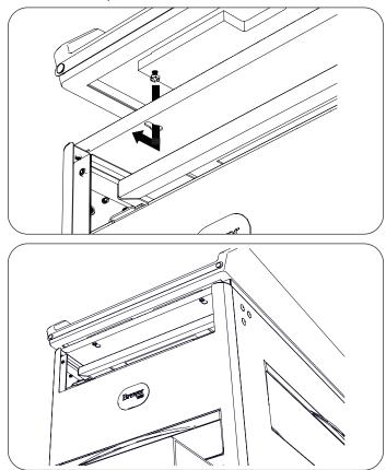
2. Fasten rear screws thru the mounting plate and in to the pediatric top at the rear of the table.
