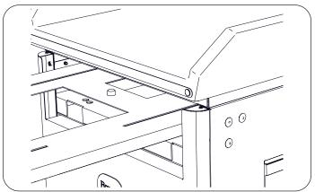
4. Insert debris pan and drop in toe board.
