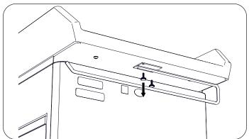
5. Loosen the pediatric top front hex screws and remove rear screws. Slide pediatric top towards the rear of the table so the front hex screws can clear the keyhole openings in the mounting plate. Remove the pediatric top.
