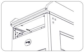
4. Remove paper roll holder by unscrewing the two round thumb screws.
