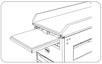
5. Fasten paper roll holder in desired orientation with round thumb screws.
