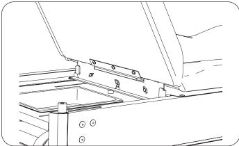
5. Install new leg extension pad, making sure curved edge faces the rear of the table.
