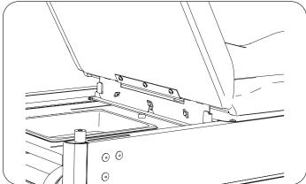
7. Install new leg extension pad, making sure curved edge faces the rear of the table.
