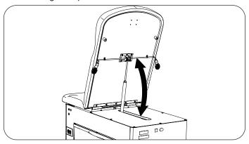
11. If you have a paper roll holder, attach it in desired orientation with two round thumb screws. Use new round thumb screws if needed.
