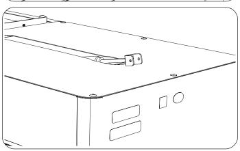
3. Remove end two thumb screws, then loosen, but do not remove center thumb screw.
