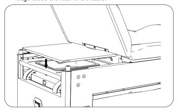
6. Raise the cylinder up into the seat bracket located on the back surface of the backrest.
