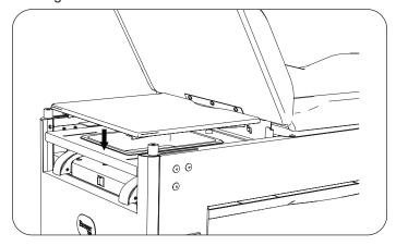
8. Raise the cylinder up into the seat bracket located on the back surface of the backrest.
