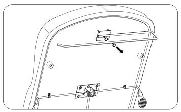
2. Remove the upper gas cylinder cotter pin and clevis pin.
