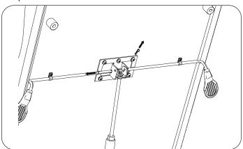
3. Rest gas cylinder on top cover plate.
