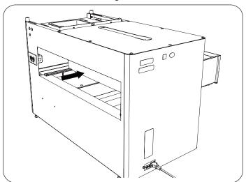
2. Reach through drawer opening and attach lower gas spring with clevis pin and secure with cotter pin. Rest the upper end of gas spring on top panel.
