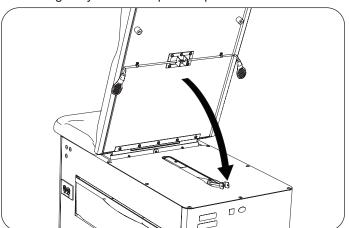
4. Lower back upholstery and raise seat. Remove two end thumb screws and loosen but do not remove center thumb screw.
