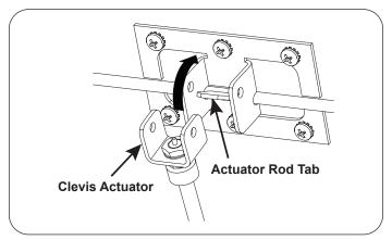
Insert the clevis pin through the actuator clevis and seat bracket making sure the tab on the actuator rod is between the clevis pin and top of the cylinder. Insert cotter pin into clevis pin.
