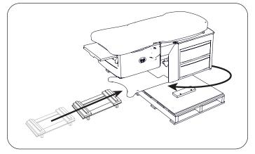
10. Move table to its final location. Lift off of furniture dolly and set down into position. Do not push or pull sideways on fully extended leg support when positioning table.
