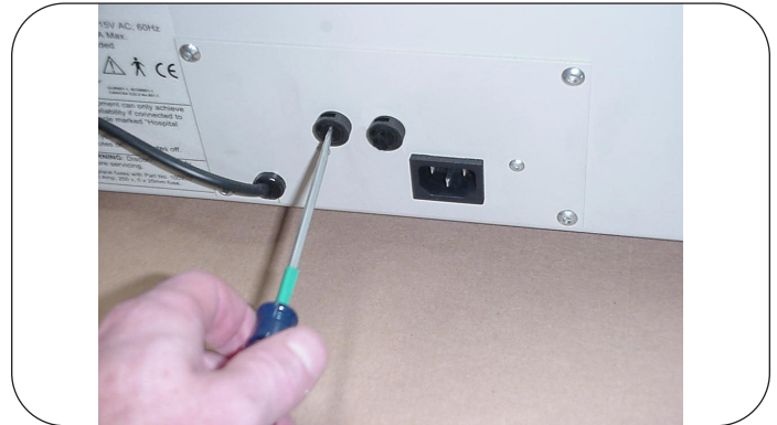
Figure 53. Tables with drawer warmer and no outlet use two 1A fuses
