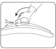
Backrest assembly may now be reattached to Control Plate with Handknob. The order of the washers on the Handknob is important-see diagram on far right.
