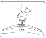
4. Rotate Backrest Upright Bar in other direction to allow other side of the Hinge Pin to pass through other hole in mating bracket. Note: pin may need to be pushed in to clear the edge of the mating bracket.
