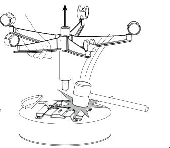
3. Place protruding portion of cylinder over wooden block and strike with mallet until it releases. Repeated blows with the mallet will be required to cause release. Note: striking the base in different spots around the cylinder will help to ease release.
