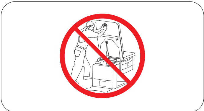
Figure 13. DO NOT Push on Backrest
