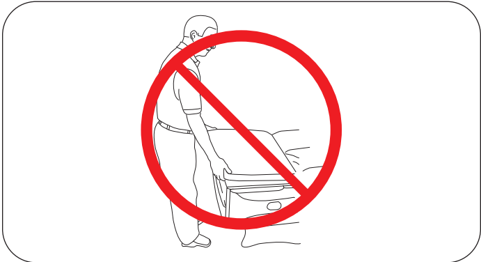
Figure 12. DO NOT Lift by Upholstery
