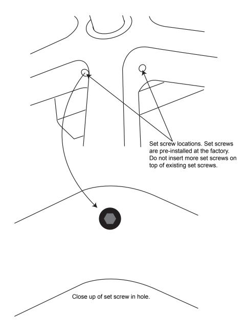
**Important!** Make sure that both set screws in the caster base are tight to the upright pole. If set screws are not tight the pole will be wobbly and can turn inside base causing wires to twist and separate.
