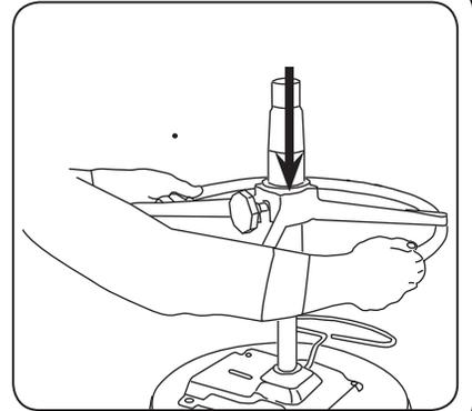
3. Wipe excess moisture from cylinder if it had been dampened, and raise and lower the footring until it begins to grip the cylinder.
