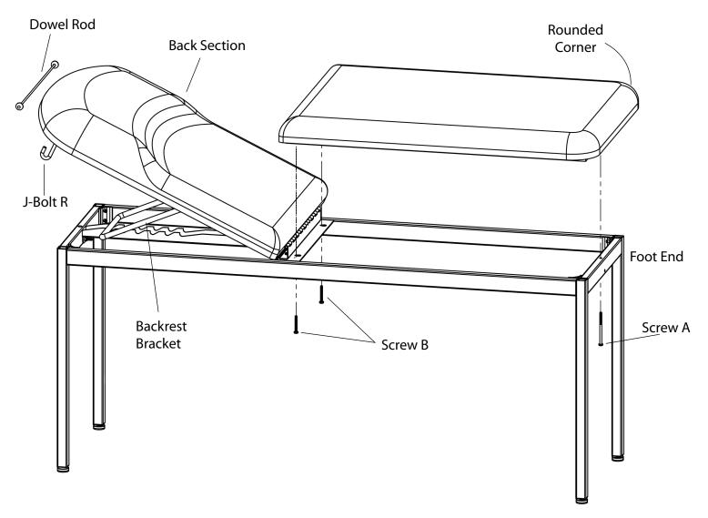
STEP A: Rotate Back Section until Backrest Bracket is engaged or top is horizontal on frame.
