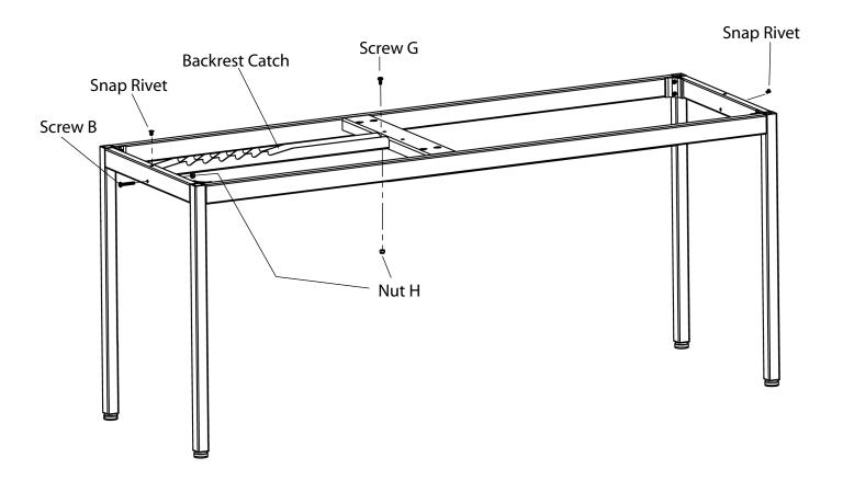
STEP A: Install Backrest Catch as shown in the drawing above.
