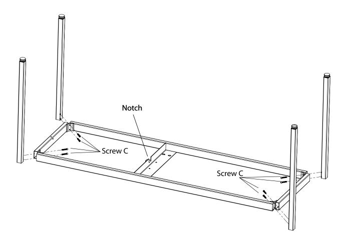
STEP A: Start with table frame inverted: note the position of the Notch in the drawing above is facing upwards.
