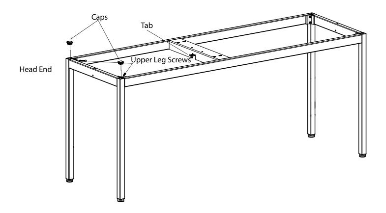
STEP A: Remove 2 Upper Leg Screws at Head End of the Table, one on each of the two legs. (See illustration above.)
